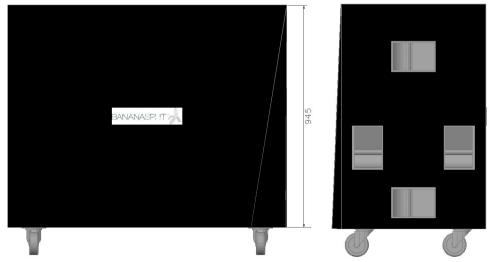
Drop over cover for a d&B Audio Technik B2 Sub & E7911 Lid. Overall Unit size 1160mm x 940mm x 580mm high. Make Covers Internal dimensions 1180mm x 600mm x 945mm high.
