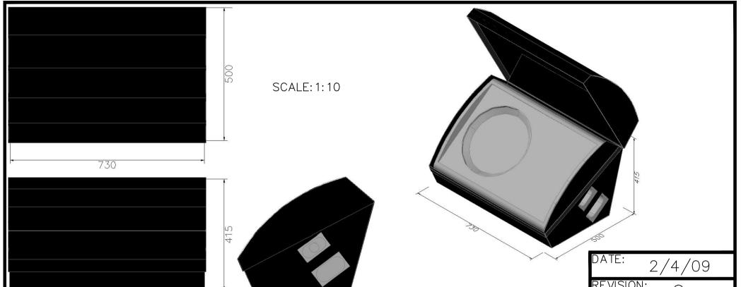
Fully Enclosed Transit Wrap for a Turbosound TFM-450 Speaker. Overall Unit size 538mm x 371mm x 711mm high. Make Wraps Internal dimensions 730mm x 500mm x 415mm high Overall. Black Nypad bag, top opening only, secured by Velcro flaps. Cut outs on side for access to unit handle. Plastic reinforcement in lid over speaker face only.
