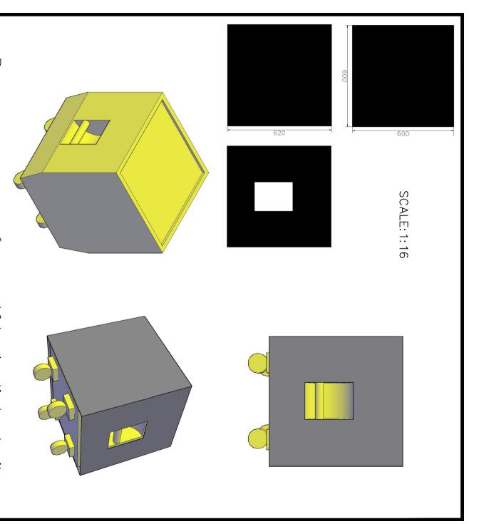
620mm high. Make covers Internal dimensions 600mm x 600mm x 620mm high. Black nypad speaker. Cut outs on sides to allow access reinforcement over speaker face to protect bag, open at base to fit over unit. Wood Drop C4-SUB. Unit size 580mm x 580mm x handles. Room for print on front. over cover for a d&b Audiotechnik
