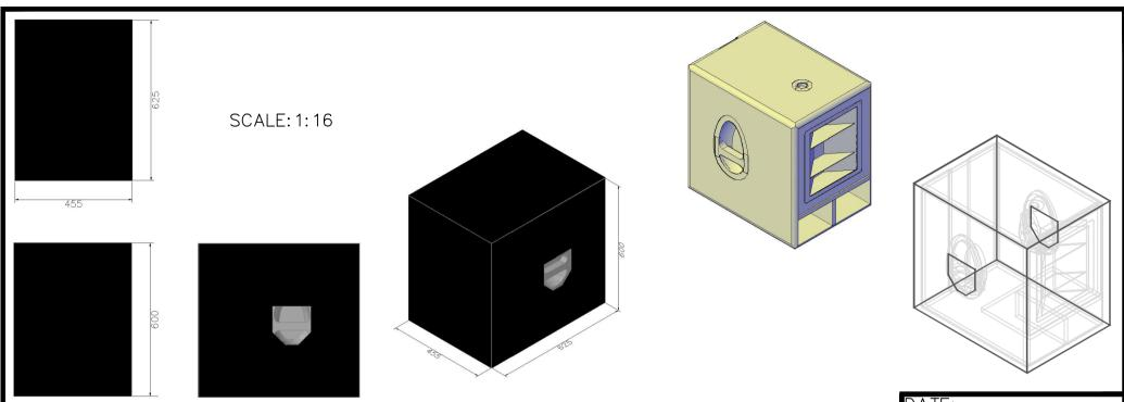
Drop over cover for a Mackie SWA1501 Active Subwoofer System. Overall Unit size 436mm x 603mm x 600mm high. Make Covers Internal dimensions 455mm x 625mm x 600mm high.
