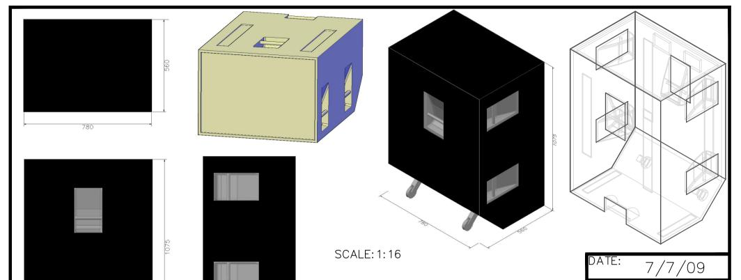
Drop over cover for an EAW SB1002 Speaker. Overall Unit size 760mm x 542mm x 1071mm high. Make Covers Internal dimensions 780mm x 560mm x 1075mm high Overall. Black Astropad cover, open at base to fit over unit, and shaped around base to give access to wheels and lower handle. 6 cut outs for access to unit handles, 2 on each side and 1 on both front and back panels. Room for Print on Top.
