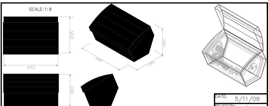
Fully enclosed Transit Wrap for an L'Acoustics MTD 108a Speaker. Overall Unit size 250mm x 241.5mm x 421mm high. Make Covers Internal dimensions 440mm x 295mm x 260mm high Overall.
