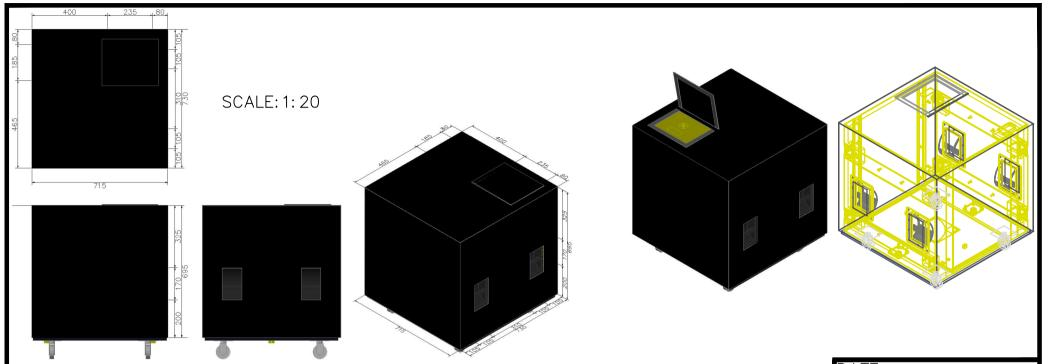
Drop over cover for an L'Acoustics DV Sub Speaker. Overall Unit size 695mm x 724mm x 708mm high. Make Covers Internal dimensions 715mm x 730mm x 695mm high.
