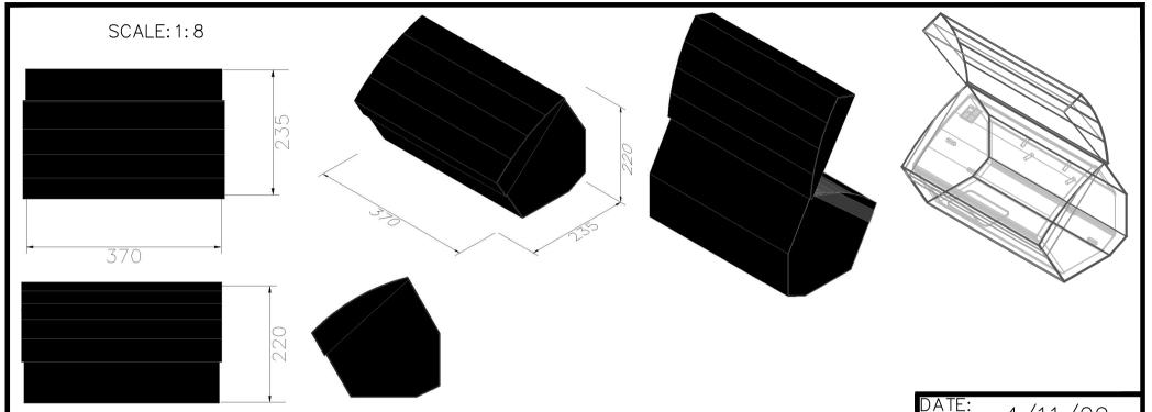
Fully enclosed Transit Wrap for a d&B AudioTechnik E3 Speaker. Overall Unit size 190mm x 204mm x 352mm high. Make Covers Internal dimensions 370mm x 235mm x 220mm high Overall. Black Nypad cover, top opening only, secured by Velcro flaps. Plastic reinforcement in lid, over speaker face. Room for print on lid if required.
